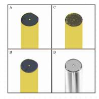
Figure 1: Images of TSP025375 cut by different methods. A) Standard Cleave, B) Precision Cleave, C) Saw Cut & D) Laser Cut.
